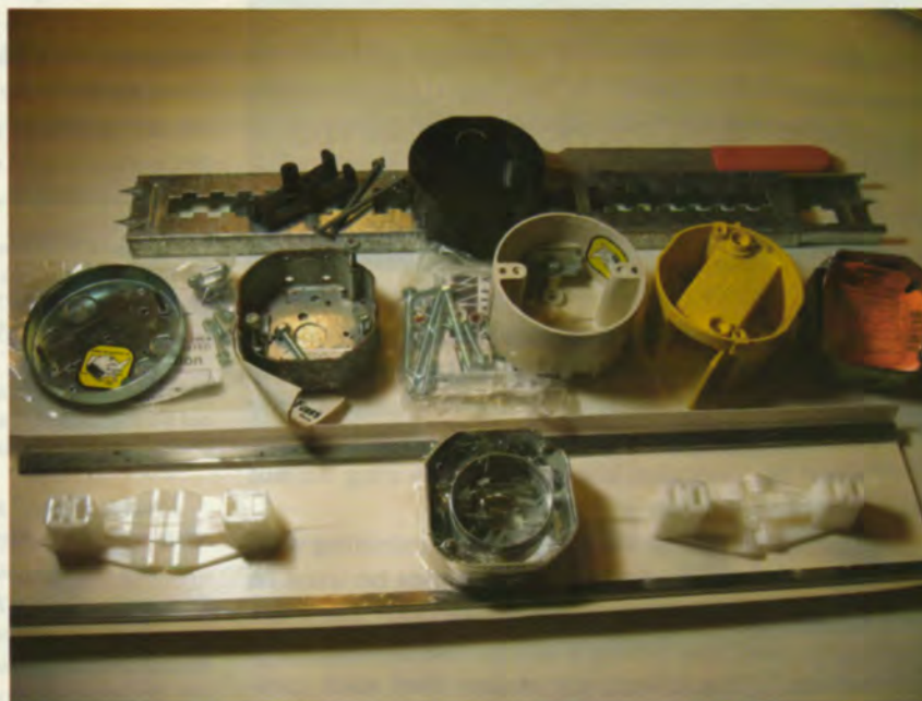
Photo 4. These outlet boxes have been specifically listed for fan support. The one in back comes with hardware to allow it to be supported between joists without removing the ceiling finish. The yellow one at center right is quite ingenious in terms of accounting for required wiring volume in a fan box intended for the bottom edge of a ceiling joist. The ceiling pan to the left has a volume of 8 cu. in., and the kit at the bottom is listed for use in a suspended ceiling.
